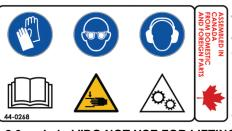
44-0268: This label is located on the winch housing. It contains the safety icons and should be cleaned or replaced if it becomes dirty, damaged or torn off.
